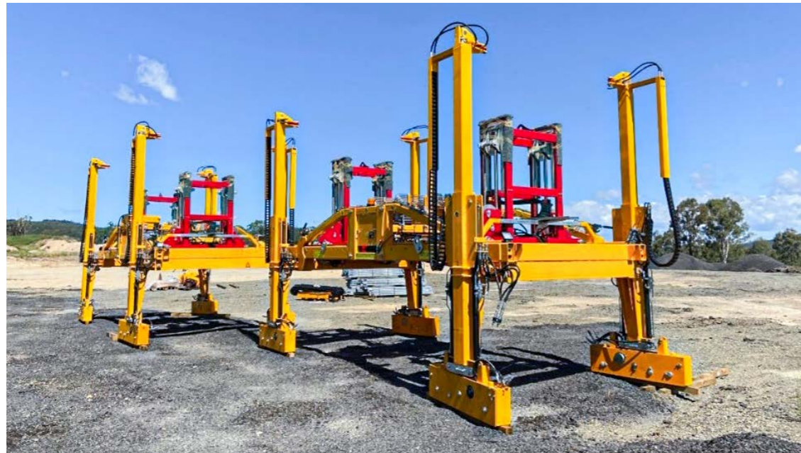
Two rail or wheel bound remote controlled mobile gantry cranes designed to lift and place the 7.5 tonne floating slab track units to be used on the Cross River Rail project.
